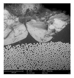
The larger items in the picture are grains of sand. It has been recognised in many research papers that sand coated BFRP bars results in an increased bond strength to the surrounding substrate.
