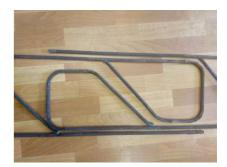
Currently there is no BS or EN for Basalt FRP bars for reinforced concrete, however we do have a National Technical Certificate and certification to ASTM D7957 which can be viewed here (hyperlink)
